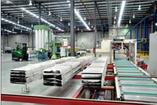
Figure 5. Profiles are automatically bundled and ready for packing.
